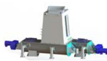
Metering screws (divide the fuel flow for different lines)
